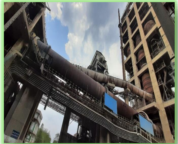
Design: 6000 TPD; Operating 8000 TPD; 5 Stage ,2 String ILC Kiln 4.75 mØ x 74m L Cooler SF 4x6 F
